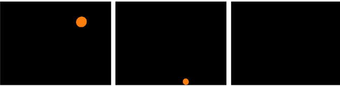
Fig. 6. Masked images of the free falling ball at time step 1 (left), time step 2 (middle) and time step 3 (right). These images show how the ball enters the view of the camera and then leaves.
